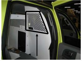
Position <sup>1</sup>/<sub>4</sub>" lexan shield Using holes in partition mark and drill shield Attach using <sup>1</sup>/<sub>4</sub>" x <sup>3</sup>/<sub>4</sub>" carriage bolt and serrated nut
